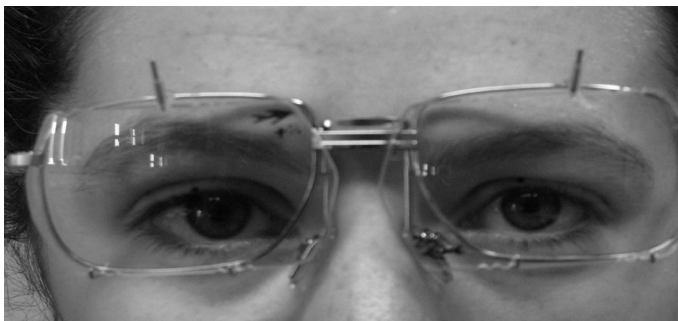
Figure 1. Custom frames made to allow custom lenses, including grooves to allow for horizontal adjustment of interpupillary distance and a centre lever on the nose-piece for standardised movement of the viewing zone 12 mm below the optical centre (Ralph Clarke Optical, Castle Hill, Sydney).
